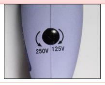
In this image, you can see that some appliances have a switch for use between higher and lower voltages. This can be used overseas with only a **plug adaptor**, but don't forget to flip the switch!
