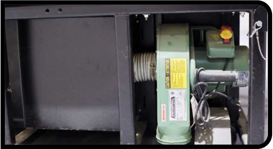
Figure 27: Dig box dust extraction system
