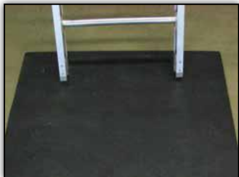
Figure 2-8. Base of the ladder should be on a non-slip mat.
