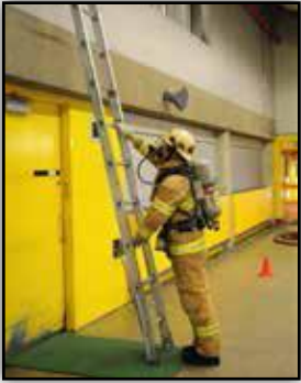
Figure 3-7. 3.6 m (12 ft) ladder in the final raised position.
