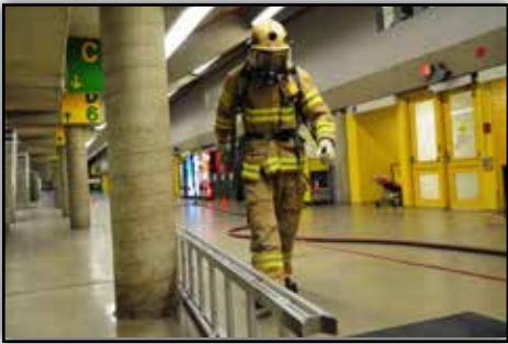
Figure 2-2. View of 3.6 m (12 ft) ladder starting position. Alternately, the ladder can also lay flat on the floor.
