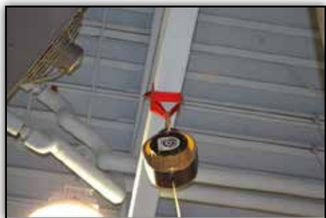
Figure 2-10. View of an auto descender attached over the ladder.
