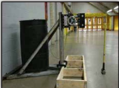
Figure A. The forcible entry device, home-made stand, barrel, wooden footplate, and sledge hammer set up and ready for use. Two 6 ft lengths of 2" x 6" connected together with four 2" x 6" x 15" cross-braces to form a foot stop barricade that can be attached to the bottom of the unit with "C-clamps" to prevent firefighters from moving past the front plane of the unit.
