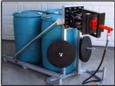
Figure B. The forcible entry device mounted using the stock stand available through CPAT Distribution, Inc. The forcible entry device is in the process of being calibrated.
