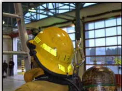
Figure 2-11. View of the firefighter with the auto descender attached to the harness via the O-ring on the back, close to the firefighter's neck.
