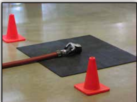
Figures 2-4 and 2-5. General view of the set-up for measuring the force required to move the charged 45 mm hose 30.48 m (100 ft).
