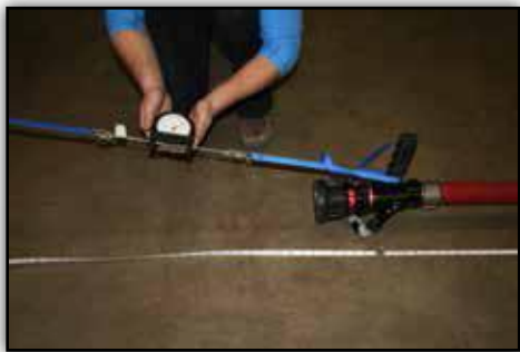
Figures 2-4 and 2-5. General view of the set-up for measuring the force required to move the charged 45 mm hose 30.48 m (100 ft).
