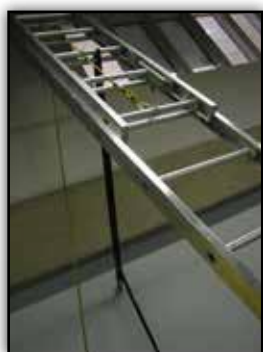
Figure 2-9. Anchor strap from the 10 th rung to an “eye-bolt” on the wall.
