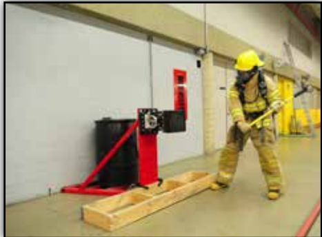
Figure 2-14. View of the set-up for the ALCO Forcible Entry task.
