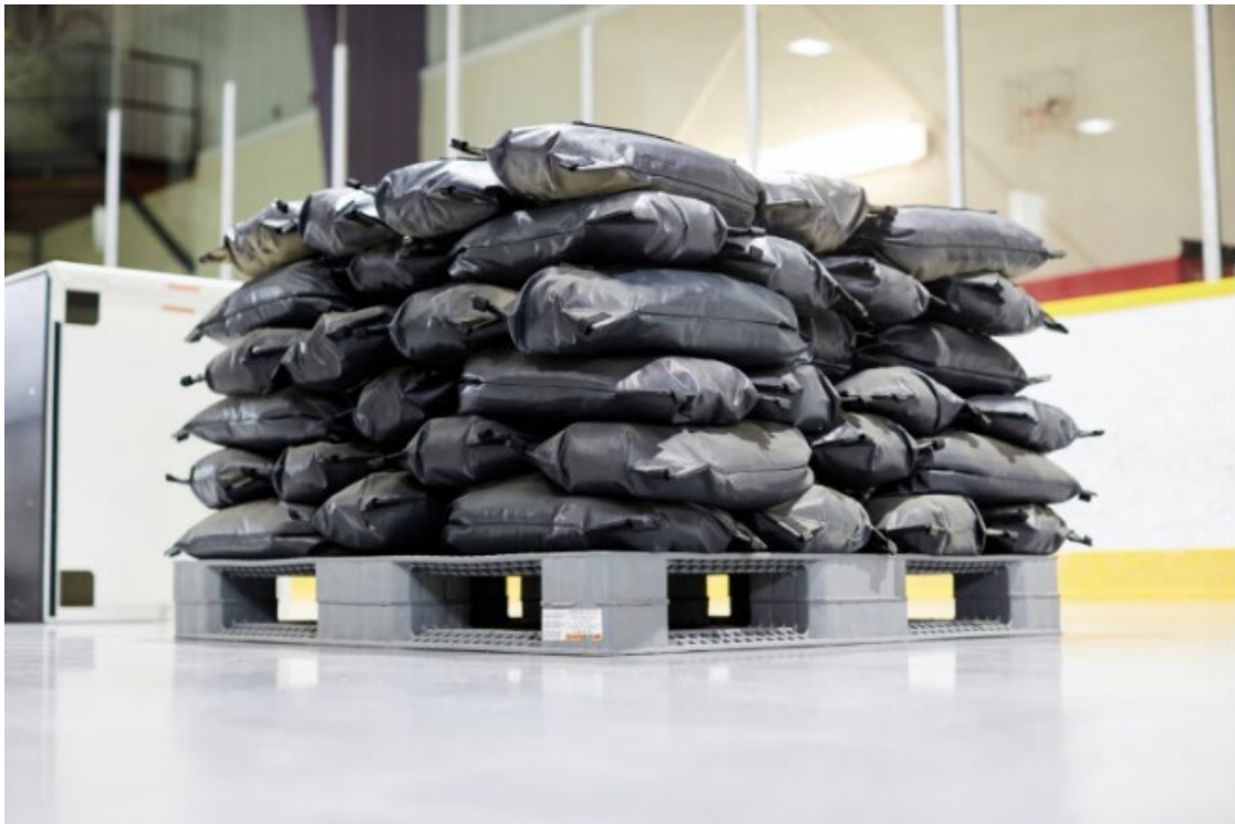
Figure 41: Alternate layers of sandbags
