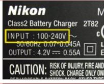
Most electronic devices have a prominent label that looks like this picture. On this device (a camera battery charger), you can see that after "Input" it says "110 – 240V", which means that it can be used with any voltage within that range, including the 110V standard in Canada or the 220-230V standard in much of Europe. All you will need is a plug adaptor.
