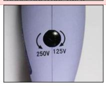
In this final image, you can see that some appliances have a switch for use between higher and lower voltages. This can be used overseas with only a **plug adaptor**, but don't forget to flip the switch!
