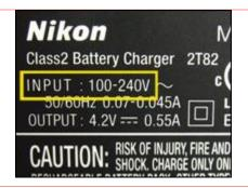
Most electronic devices have a prominent label that looks like this picture. On this device (a camera battery charger), you can see that after 'Input' it says '110 - 240 volt', which means that it can be used with any voltage within that range, including the 110 volt standard in Canada or the 220-230 volt standard in much of Europe. All you'll need is a plug adaptor.
