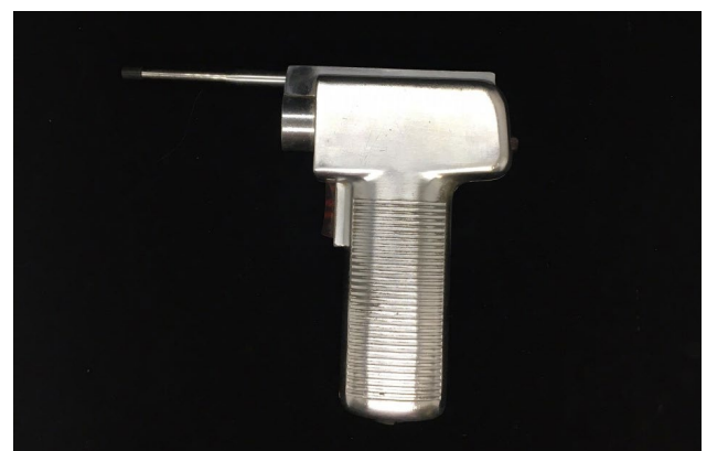
A light gun was used with the original computer system, SAGE, in the Underground Complex. Photo credit: CFMAD photo
